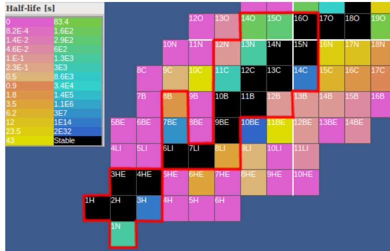
Figure 2.2: Cut from the nuclide chart, nuclides framed in red are those considered in the PARthENoPE code, (credit: www-nds.iaea.org ).
