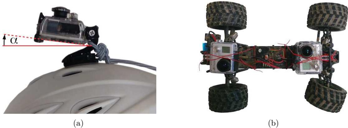
Figure 4.1: The figure shows the two experimental setups used to record the training and test data. (a) One camera (either UV or RGB) is mounted on a helmet with a tilt angle  $\alpha$  above the horizon. The track has been recorded using both the UV and the color camera for varying tilt angles  $\alpha \in \{-30^\circ, -20^\circ, \dots, 30^\circ\}$ . (b) Both cameras are mounted on the RCC, allowing us to record the same run with both cameras simultaneously.
