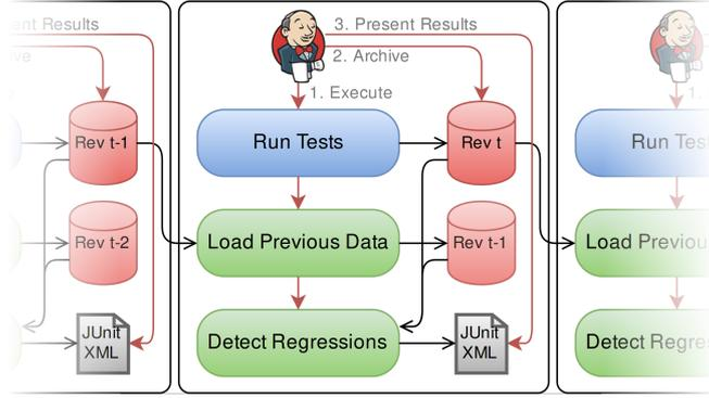
**Figure 6.** Integration of the testing framework in the Jenkins CI server. Each black rounded box represent a single Jenkins build and therefore execution of the tests for a component. Time and component versions progress from left to right.
