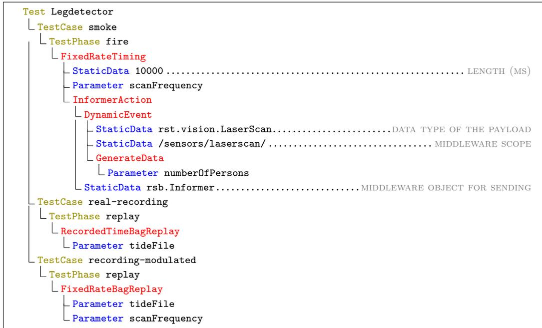
**Figure 3.** Structure of a performance test for a component which detects legs in laser scanner readings. The test consists of three distinct test cases, each with a single test phases. The general test case and phases structure is marked in olive green, actions are marked in red and data-related actions are marked in blue.
