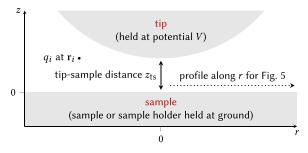
FIG. 1. Schematic view (not to scale) of the considered model for the probe tip and the flat sample. The spherical tip (which is not shown completely) is laterally centered at r=0 and at a distance of  $z_{ts}$  above the sample surface, which is located at z=0. A set of point charges  $\{q_i\}$  at position  $\{\mathbf{r}_i\}$  can be placed in the tip-sample system.
