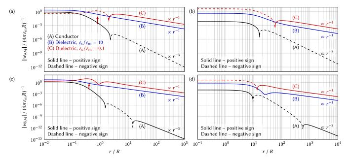
FIG. 5. Profile of the weight functions as a function of the lateral distance r for charges at a fixed height of z = R/100 above the sample. The AM-KPFM weight function is shown in (a) and (b), while the FM-KPFM weight function is shown in (c) and (d). In the left column [(a) and (c)], the tip-sample distance is  $z_{ts} = R/40$  and in the right column [(b) and (d)] the tip-sample distance is  $z_{ts} = 10R$ .
