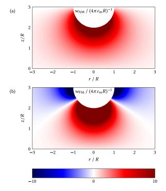
FIG. 2. Weight functions for case (B) with a tip-sample distance of  $z_{\rm ts} = 2R$ . The AM-KPFM weight function is shown in (a) and the FM-KPFM weight function in (b). The sample surface is located at z=0. The color bar shown below applies for both plots.
