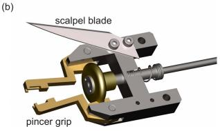
FIG. 5. (Color online) (a) Wobble stick with attached scalpel blade. (b) Drawing of a scalpel blade attached to the frame of the pincer grip of the wobble stick (Ref. 6) which is part of an *in vacuo* transfer system.
