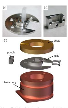
FIG. 1. (Color online) Sample holder for system 1. (a) Inlay plate with incorporated clamping mechanism. (b) Steel pouch for sample crystals. The three screws facilitate precise force adjustment. (c) The inlay with the clamping mechanism is assembled between the copper base body of the sample holder and the chute for the approach of the beetle type scan head.
