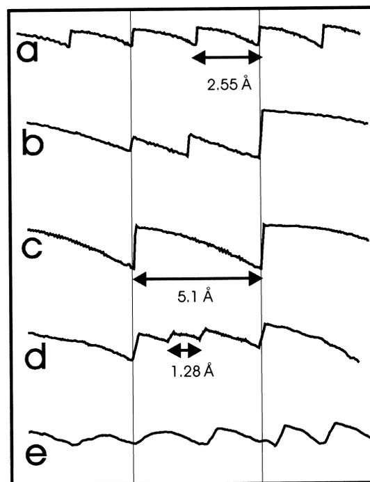
Fig. 3. Various tip height curves illustrating the artificial diffusion dynamics of a molecule along the close-packed row directions of Cu(111) during the lateral manipulation process: single copper-atomic-site hops (a), mixed single and double copper-atomic-site hops (b), double atomic hops (c), mixed ‘hop-scotch’, single and double copper-atomic-site hops (d) and sliding and pulling (e).
