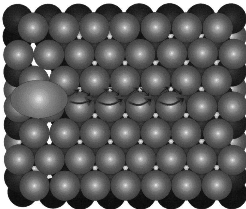
Fig. 4. Schematic drawing illustrating the possible diffusion paths of diiodobenzene along the Cu(111) close-packed rows. The curved arrows demonstrate the single copper-atomic-site hops in which the molecule will jump to only hexagonal close-packed (hcp) or face-centred cubic (fcc) sites. The zig-zag arrows demonstrate 'hop-scotch' motion in which the molecule will visit both fcc and hcp sites.
