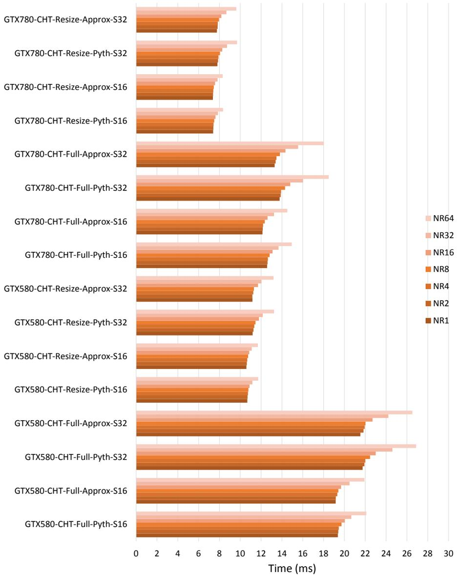
Figure 6.10: GPU computing performances for configurations using CHT algorithm.
