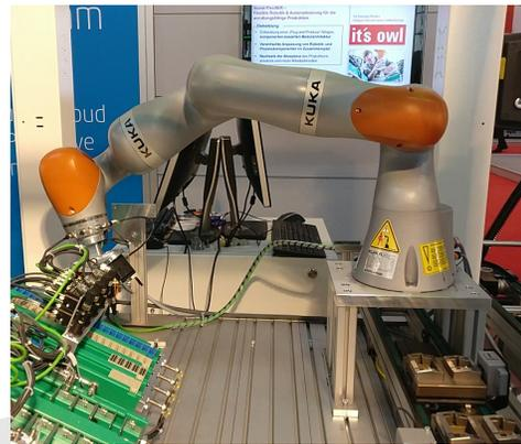
*Fig. 1: Modular production system with a collaborative robot during an assembly task on the Hannover Industry Fair in 2017.*
