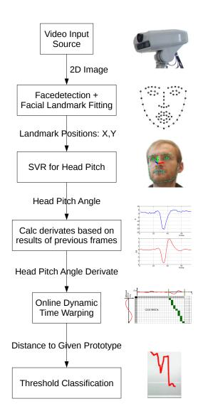
Fig. 3. Nod Detection System Overview
