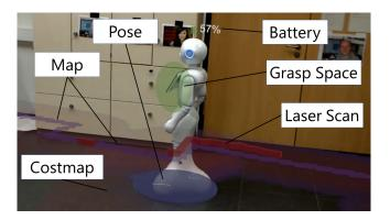
Figure 1: The sensory data which are visualized in the HoloLens: Map, costmap and laser scans, the robot's pose and battery status. Additionally, the space where the robot can grasp objects is shown.
