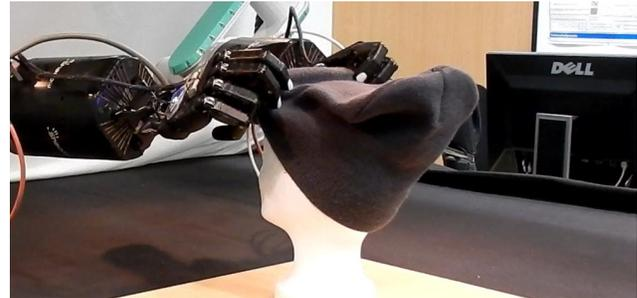
Fig. 1. A robot putting a knit cap on a styrofoam head.
