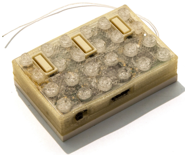
Figure 4.11: Case design III for the BRIX 2 base module.
