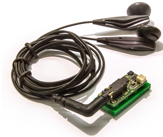
Figure 5.10: Opened BRIX 2 AudioAmp Extension Module connected to earphones.
