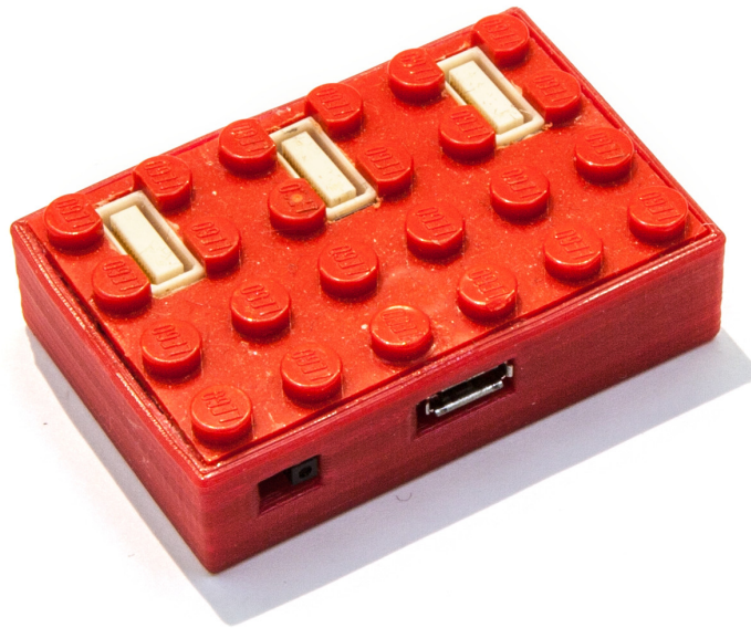
Figure 4.9: Case design II for the BRIX 2 base module.
