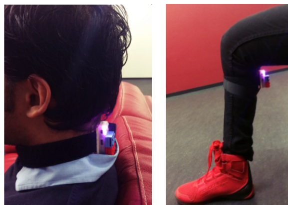
Figure 6.16: BioSense module placement: Sensors and actuators are mounted on the neck and the lower leg of the user.
