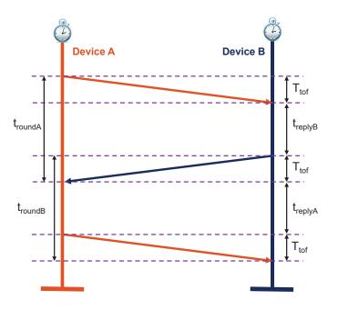
Fig. 1. Illustration of Double-sided Two-Way Ranging Method
