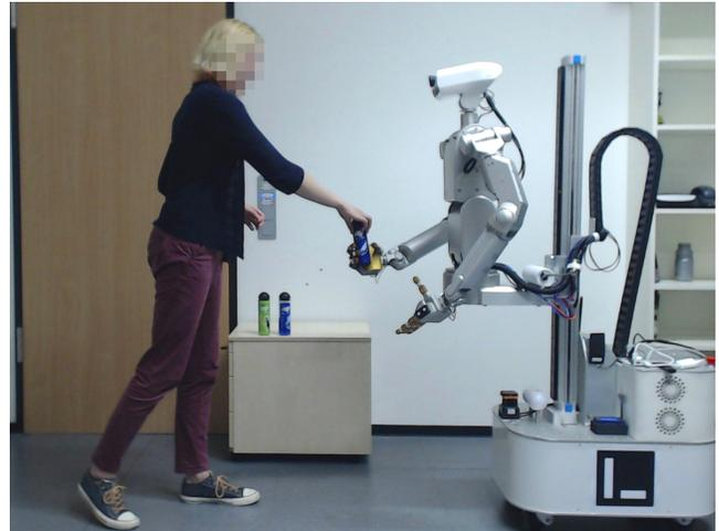
**Figure 1: Human-Robot Handover Experiment: The participant takes one of the objects from our robot Floka. A gesture with the left hand of the robot aims to improve synchronization between human and robot.**
