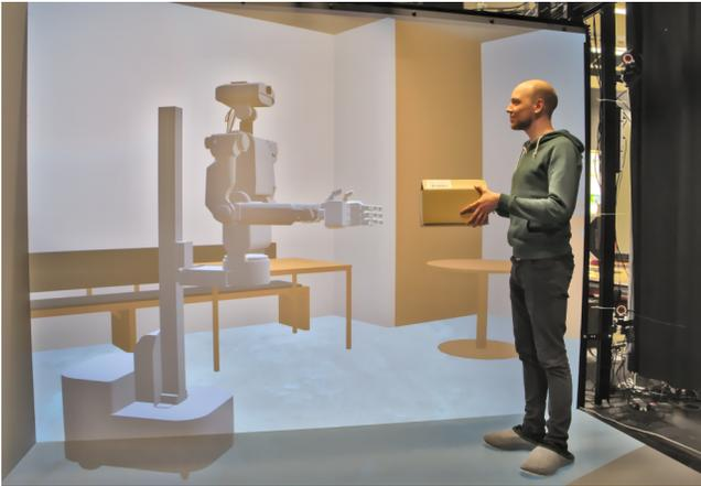
**Figure 4: A virtual Floka displayed in the CAVE is receiving an object from Patrick. For the picture stereo was disabled and the perspective was corrected for the camera and not the interacting user.**
