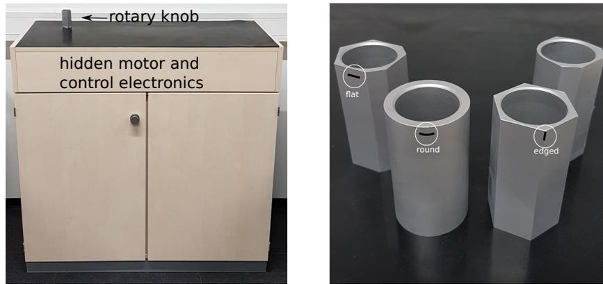
**Fig. 1.** *Left:* The *Twister* front view. The current design of *Twister* in a form of a cupboard aims to hide the extensive control electronics and motor from the participants in case the rotational joint is used actively. Participants are placed behind the cupboard during the experiments. The apparatus can be separated into two parts, the top and the bottom, in case the height needs to be adjusted manually. *Right:* Examples of different rotary knobs.
