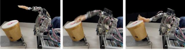
Fig. 4. Snapshots of generalized drumming action. Starting configuration  $\mathbf{q}^{\text{start}}$  is shown in the leftmost picture.
