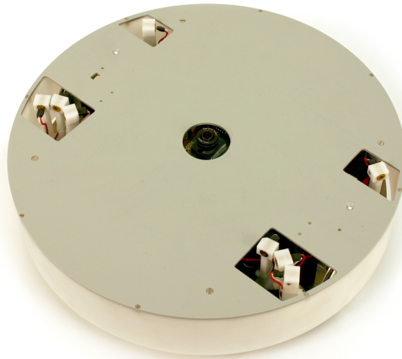
Figure 2.1.: Our cleaning robot prototype, with its outer cover installed. Our robot measures the movement of this spring-mounted cover to detect collisions (Section 2.3.2.3). The panoramic camera can be seen through a hole in the center. Furthermore, eight white pillars extend above the cover's upper lid. Each pillar contains a laser diode, which is used for obstacle detection (Section 2.3.2.2).
