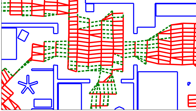
Figure 5.10.: The effect of edge classification on the map graph from Figure 5.3. Edges classified as crossing a room border are drawn as green, dashed lines. While most room-border edges are classified correctly, we also note some false-positive results within the rooms.
