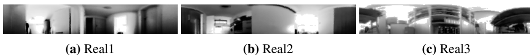
Figure 5.17.: Low-resolution, unfolded panoramic images acquired by our robot. These images are created by reprojecting, blurring and histogram-equalizing the images in Figure 5.16. In this study, we use such images to calculate the image distances from Section 5.2.2.4.
