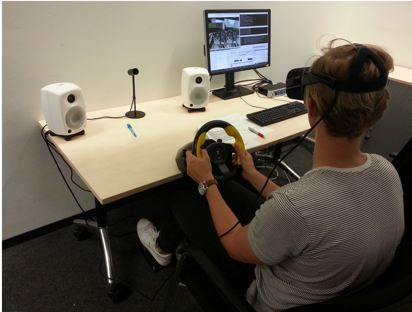
Figure 10.2.: Hardware setup for the study. Two additional loudspeakers (not seen in the picture) were placed behind the participant. The computer monitor on the right was used only for controlling the application and could not be observed by the participants during the experiment. The head tracking sensor of the Oculus Rift can be seen between the two loudspeakers in the front.
