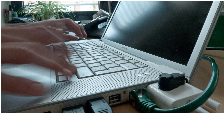
Figure 5.2.: The augmented keyboard (Bovermann, Tünnermann, & Hermann, 2010). The sounds of a user typing on a keyboard are picked up by a contact microphone, filtered, and fed back to the user. The filter parameters are determined by external data, e.g. the current temperature or humidity.
