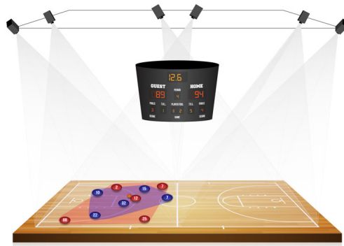
Figure 2.16: STATS SportVU system using 6 cameras at 25 fps [85]
