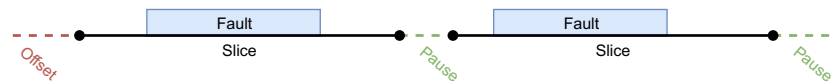
Figure 12.2: Scheduling of induced performance bugs (blue). The time of a trial (horizontal axis, from left to right) is separated into slices (black lines with round markers) with an initial offset at trial start (red dashed) and pauses between slices (green dashed).
