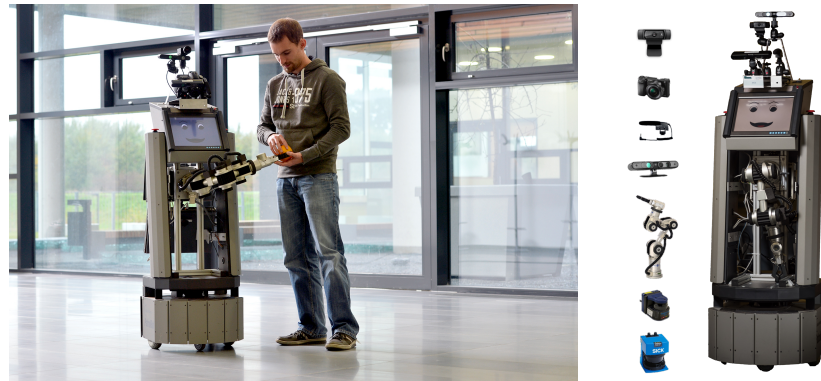
Left: ToBi interacting with a person (photo: CITEC/Susanne Freitag, reproduced with permission). Right: Sensors and actuators of the robot.
