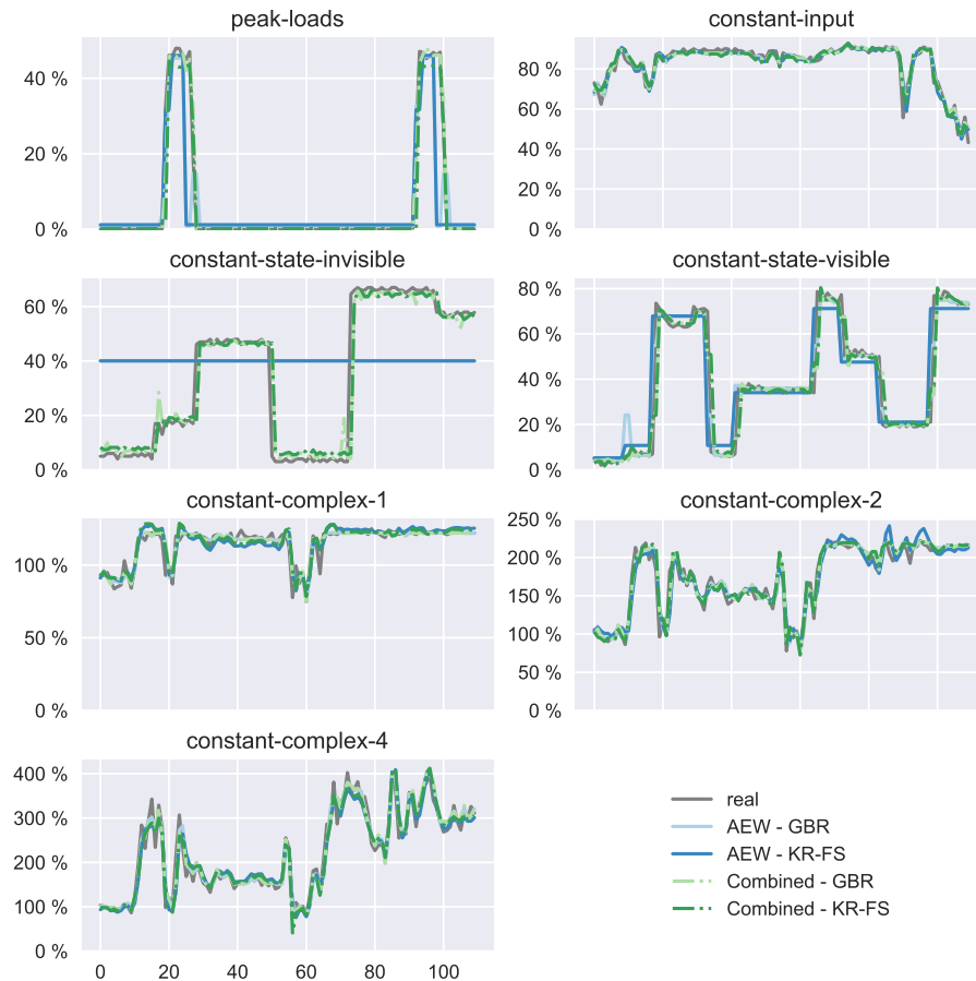
Figure 13.7: Examples for the predictions achieved for the mock components (proc/stat-utime). The unit of the y-axis is the utilization of a single CPU core in percent.
