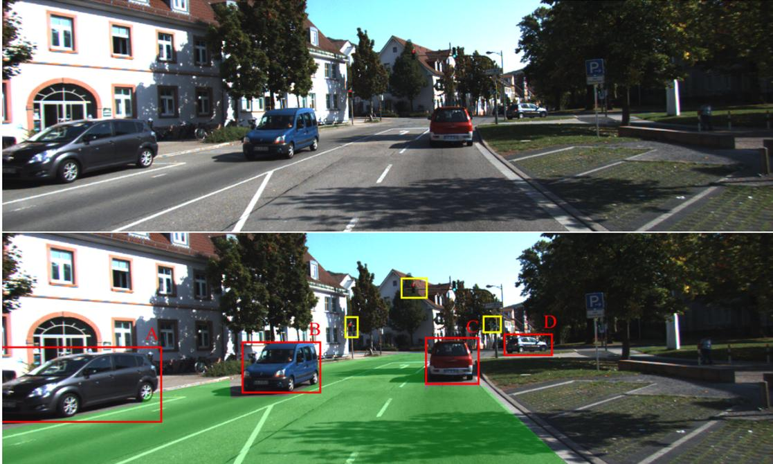
**Figure 1.2:** Typical urban intersection as seen by a camera (above). Same scene after road and object detection (below).
