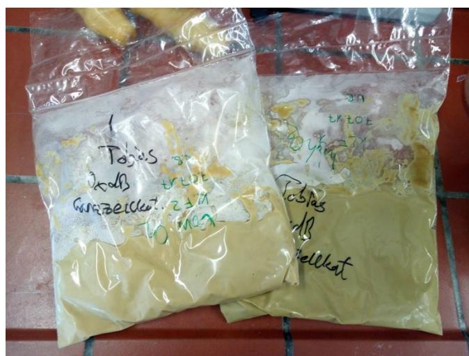
Figure 22: The obtained pellets (wet biomass) from the conducted high cell-density fermentations (left bag: Low O_2 , right bag: High O_2 ).
