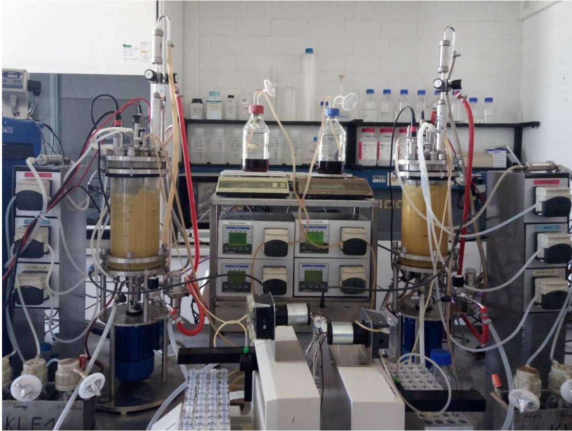
Figure 19: High cell-density equipment utilized for the overexpression of OxdB in E.coli BL21 (DE3) Codon + RIL. Left fermenter: Low oxygen level (low O 2 ), right fermenter: High oxygen level (high O 2 ).
