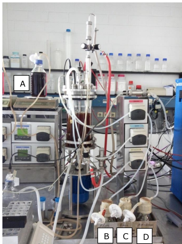
Figure 20: Bioreactor with external flasks containing feed medium (A), acid (B), base (C) and anti-foaming agent (D).
