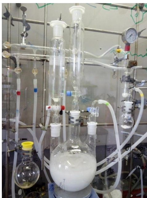
Figure 10: 2 liter scale reaction for the preparation of adipaldehyde starting from trans -1,2-cyclohexanediol.
