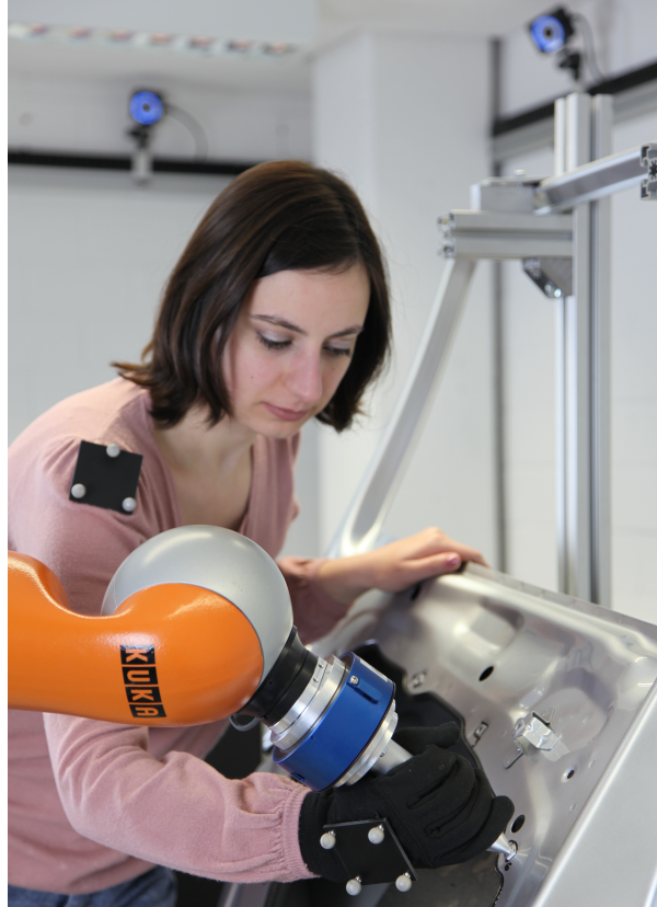
Figure 6.7: The figure illustrates the peg in the hole task, the user have to move the robot end effector into each marked drill holes in the car body.
