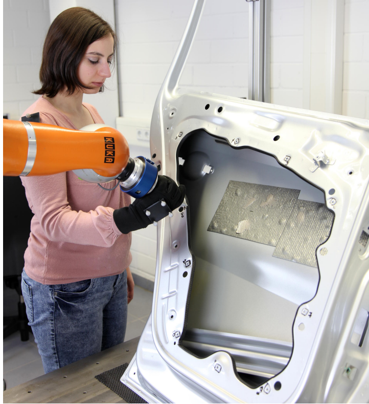
Figure 6.6: The figure illustrates the contour following task, the user have to move the robot end effector along the black rubber sealant.
