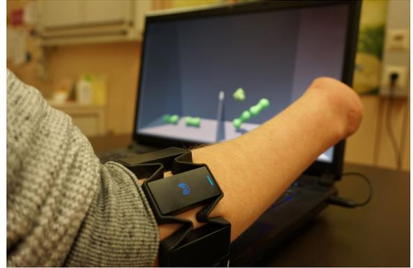
Figure 7: Study set-up: The patient is wearing the Myo armband around his forearm with the elbow resting on the table and facing the computer screen.
