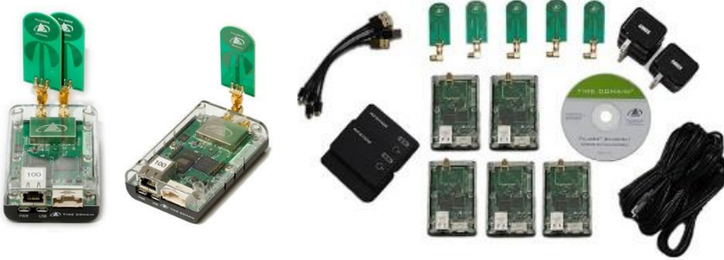
Figure 2.16: UWB products of Time Domain Company including PulsON440 (left) and PulsON330 (middle) and a development kit (right) [56]
