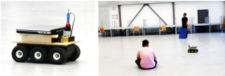
Figure 8.11: The robot platform used for the large-scale indoor experiments (left) as well as the sport hall used in these trials showing NLOS barriers (right)
