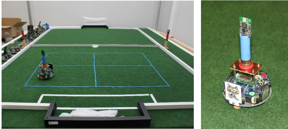
Figure 8.1: Photo of the small-scale indoor arena with the blue reference lines (left) and the development platform carrying UWB node (right)
