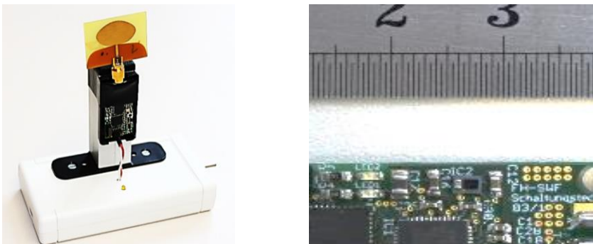
Figure 7.2: Hardware platform used for both anchor module (left) with module holder and additional backup battery and a tag module (right)
