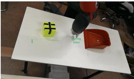
(a) Robot execution process from starting place to phase I for a cleaning task
