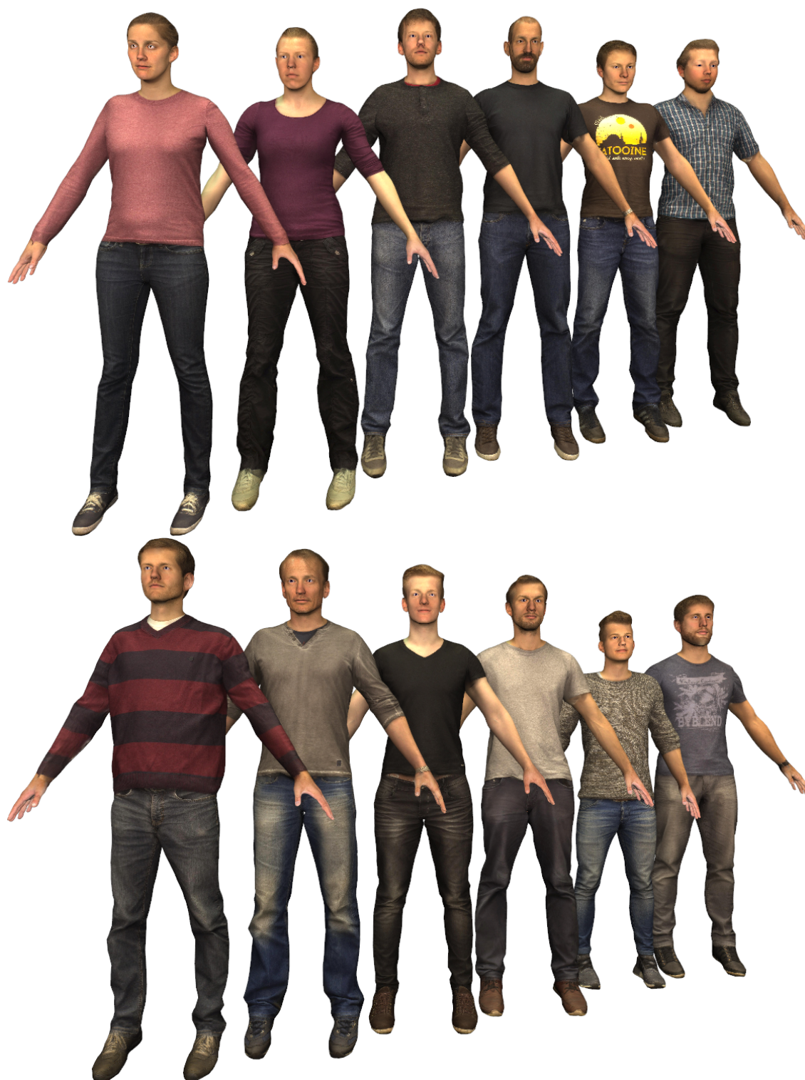
Figure 3.11: We generate realistic virtual humans from real persons through multi-view stereo scanning. The resulting characters are ready to be animated through a skeletal rig and facial blendshapes and are compatible with standard graphics and VR engines. The whole reconstruction process requires only minimal user input and takes less than ten minutes.
