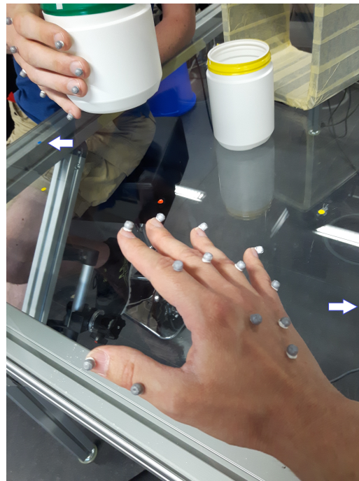
Figure 3. Photo of the experimental situation, seen from the position of the participant sitting on stool R . (Denotations as in Figure 2.) His hand with 13 reflective markers is visible in the lower center. The low number of markers is possible because of the application of inverse kinematics when determining the joint angles—see Maycock et al. [28]. The participant on stool L is visible in the upper left, the rack P in the upper right, one of the plastic cans standing in front of it. (Just for visualisation, normally, the cans are stored on an extra table behind the experimenter.) The points H_L and H_R are visible as small blue disks close to the left or right image border, respectively. (For better visualisation, white arrows pointing to H_L and H_R were added.) The points S_L and S_R are the small yellow disks next to H_L and H_R , respectively. Point T is the small red disk between them, close to the center of the picture. The situation of a direct hand-over of a small, empty can in the moment is shown, when the giver on stool L is holding the can over point T , and the receiver on stool R reaches for the can. (This would be an example of an incorrect behaviour of the participants, as a green border of the can signals an indirect hand-over. Trials like this were sorted out. In the experiment, markers were also put at the upper border of the cans.)
