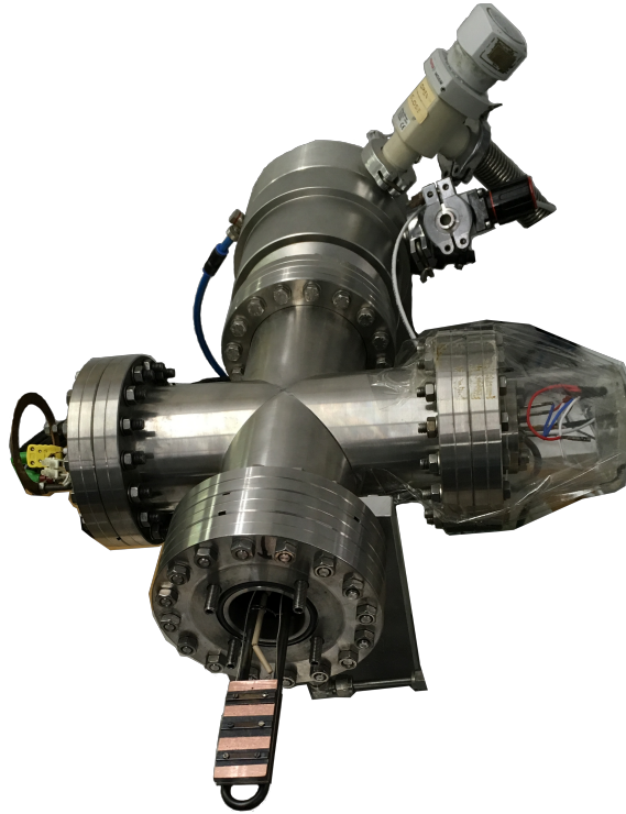
Figure 2.3 – Setup for annealing and pinning. The copper block in the front has a useable dimension of approximately 30 \times 30 \text{ mm}^2 . The samples are fixed with metal clamps for a good thermal coupling. The chamber is evacuated to 1 \cdot 10^{-8} mbar. The external magnetic field has a field strength of 5500 Oe.
