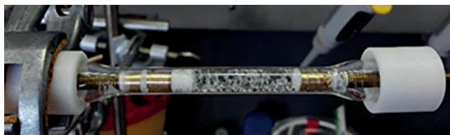
Figure 5. Picture of the packed bed reactor charged with superabsorber gel.
