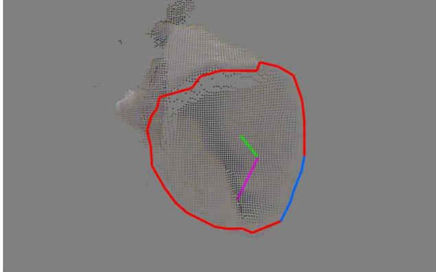
Figure 4.14: Grasp pose around the boundary of a knit cap opening. The detected boundary component is shown in red, the optimized grasp segment in blue, and the derived approach and orientation vectors in green and pink, respectively.
