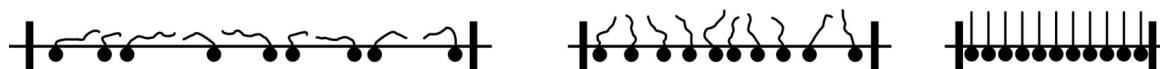
Figure 2.11: Amphiphile molecules at the air-water interface in the expanded, compressed, and closed packed state. These states are also referred to as gaseous , liquid , and solid in analogy to thermodynamics. Inspired by a Figure in Langmuir-Blodgett Films . 102
