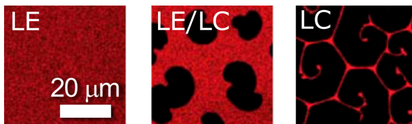
Figure 2.14: The pictures show a Langmuir film from the top view. A fluorophore (Texas Red) is conjugated to the headgroups of lipids in the Langmuir film and is distributed homogeneously (LE). During phase coexistence (LE/LC), the dye is excluded from the more-ordered LC phase, thus generating a contrast between the phases. 123
