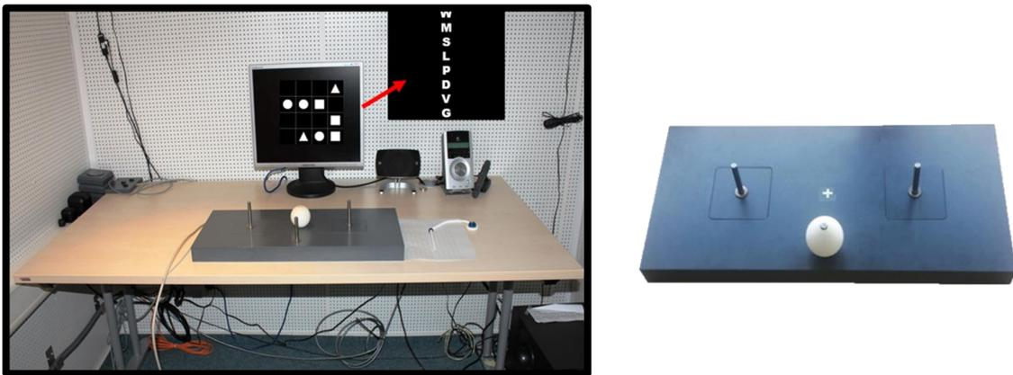
*Figure 2.1.* The experimental setup used for all the experimental studies in the current thesis. (Left) In the figure, setup includes an example stimulus for visuospatial task and verbal task and task board for manual task. (Right) Task board includes three sticks a start position (where the sphere is fitted onto) and two motor targets. Center of the task board is marked by a yellow cross.
