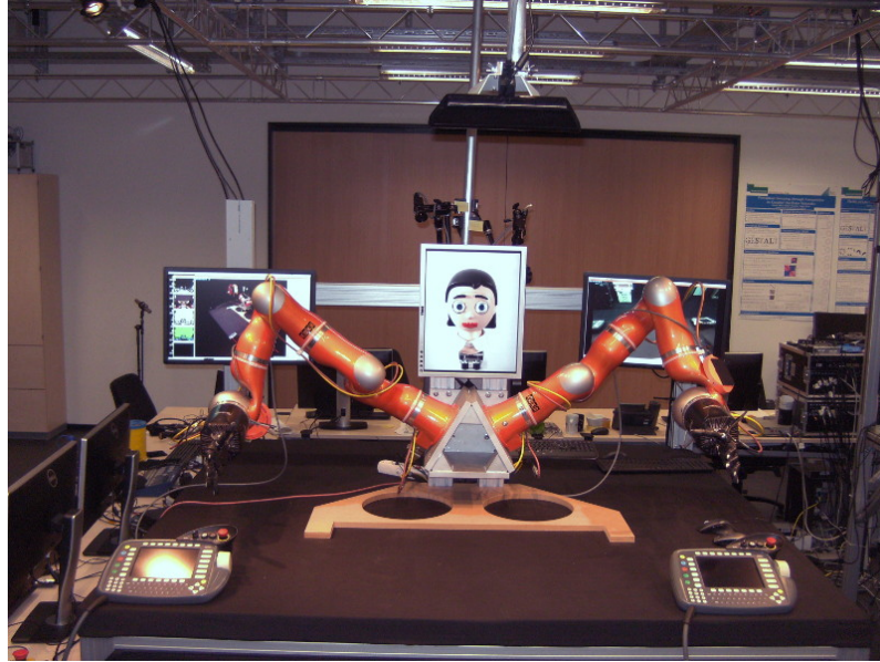
Figure 5.1: The FAMULA platform: A bimanual robotic platform supporting the investigation and development of approaches by which a cognitive system can familiarize itself with new objects and concepts through the interplay of manual action and language ( https://www.cit-ec.de/en/deep-familiarization-and-learning ).
