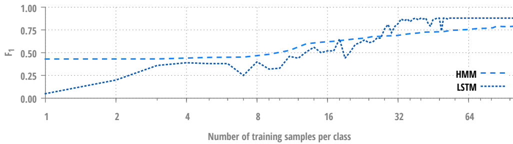
Figure 3.12: Early learning behavior, averaged over 10 random folds. HMMs outperform the LSTM network where very little training data is available, while the latter performs better with more than 28 training sequences. Note that the x-axis is scaled logarithmically.
