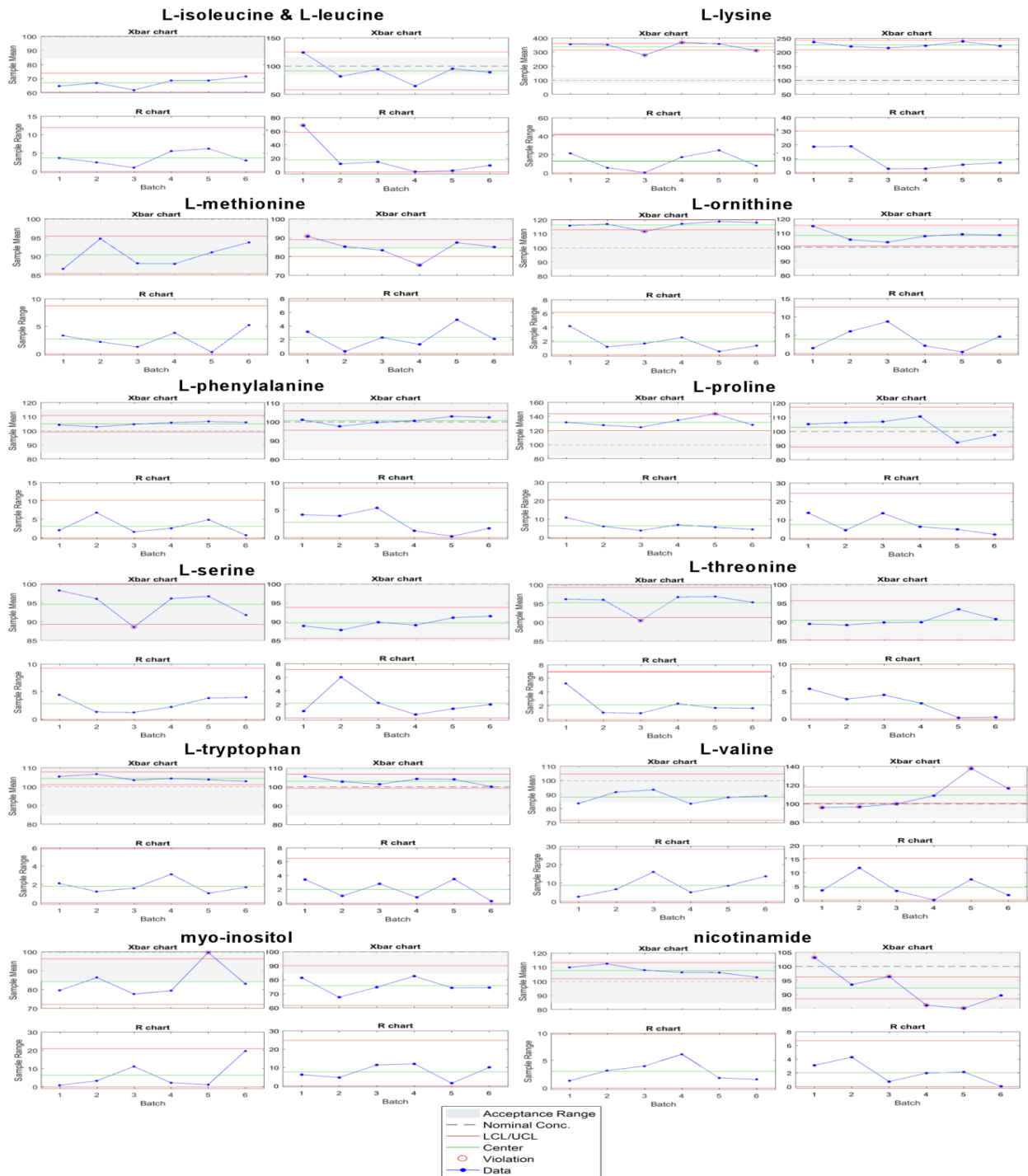
Figure 64: Control charts for compounds L-isoleucine and L-leucine, L-lysine, L-methionine, L-ornithine, L-phenylalanine, L-proline, L-serine, L-threonine, L-tryptophan, L-valine, myo-inositol and nicotinamide. The Xbar-R charts on the left of each compound shows QC samples run with batches for measuring model medium 1 preparation and the right Xbar-R chart shows the QC samples run in batches where samples from the storage stability study of model medium 2 were measured. The Xbar chart calculates if the measurement mean is in control and the R charts show if the measurement variation is in control. The dashed line symbolizes the nominal concentration expected in model medium 2 QC sample and the grey area symbolizes the \pm 15\% acceptance range. The lower control limit (LCL) and upper control limit (UCL) are automatically calculated in Matlab and show if the measured values are within the process control ranges. The green line symbolizes the center line. Violation of the control limits are shown by red circles around the blue data.
