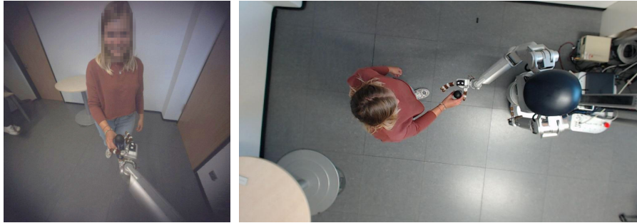
(a) Floka's eye camera looking at its hand (b) View from the top-mounted camera aligned to the interaction area
