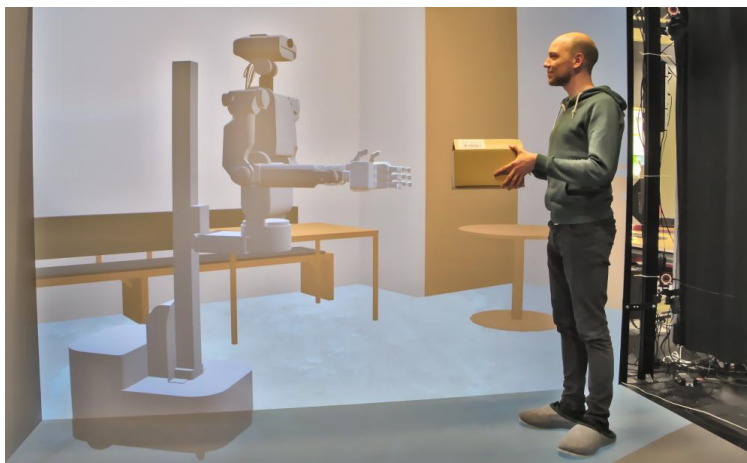
Figure 4.6: A virtual Meka M1, displayed in a CAVE, is receiving an object from Patrick. For the picture stereo vision was disabled and the perspective was corrected for the camera and not the interacting user [Mey+18].
