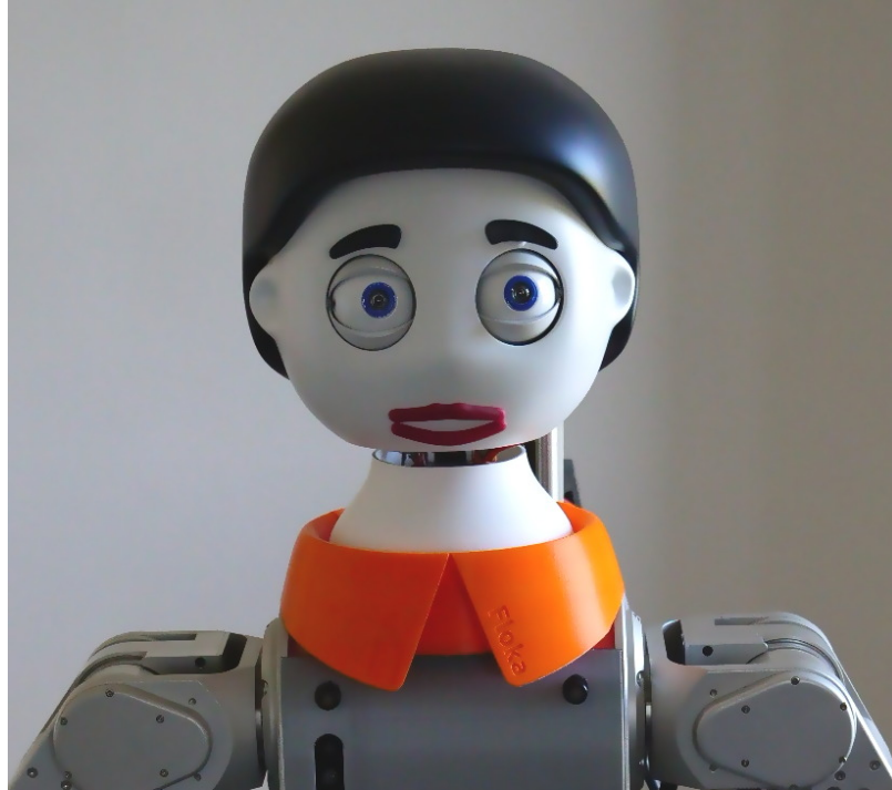
Figure 6.1: The Floka Head for enhanced gaze behaviors features two eye-balls with human-like capabilities in terms of acceleration, velocity, range of motion, and perception [SMW19]. In addition to the eyes, the brows, the lids, and the mouth are movable. The comic-character-like look increases expressiveness and allows humans to easily read emotions and gaze directions. It can be mounted on the Meka M1 to create Floka.
