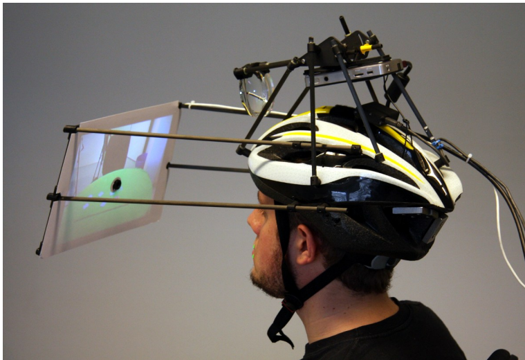
Figure 9.1.: An operator wearing the proposed bi-directional motion capture and feedback system.
