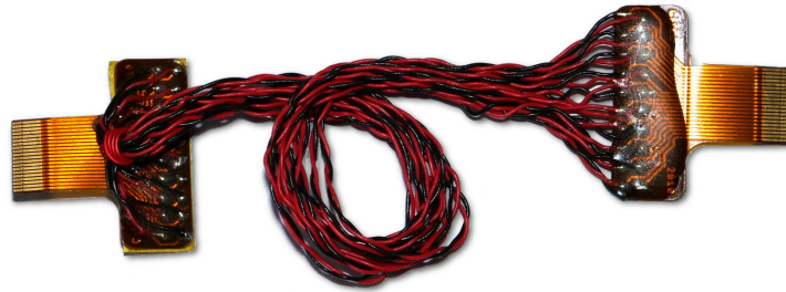
Figure 7.4.: The custom-made highly flexible replacement camera cable.
