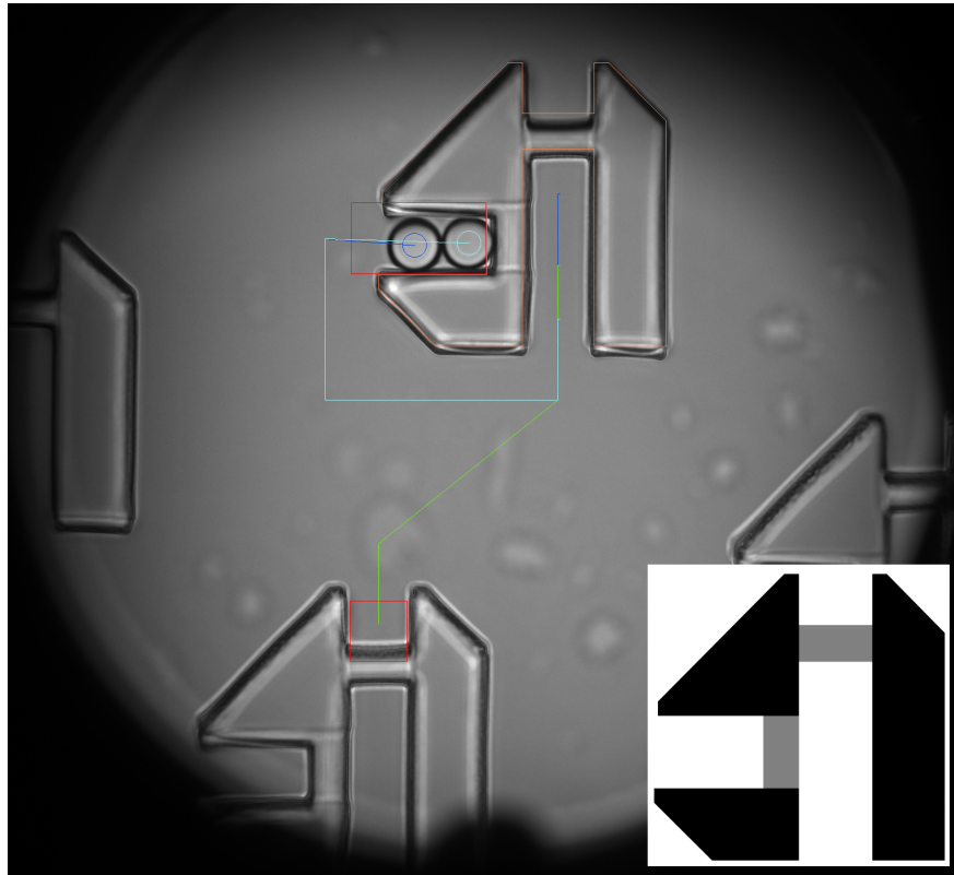
Fig. B.9.: Illustration of the measurement automation workflow. First, the trapping structure is search with the reference image (inset). The resulting position is annotated in orange. Then, in to top red rectangle, two beads are searched (blue). The bottom rectangle is checked for the presence of a cell. The left bead is then moved into the trapping structure along the dark blue path, followed by the cell along the green path and the right bead along the light blue path.
