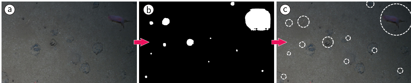
FIGURE 3. Example for inference with Mask R-CNN and the final object detection on a subsection of image TIMER_2015_09_04at09_13_31IMG_0864.jpg of the S155 dataset. The image (a) is processed by Mask R-CNN which returns a segmentation mask for “interesting” pixels (b). The regions of interesting pixels are converted to circle annotations for the final detections (c). The full image with manual annotations can be found in the supplementary material.
