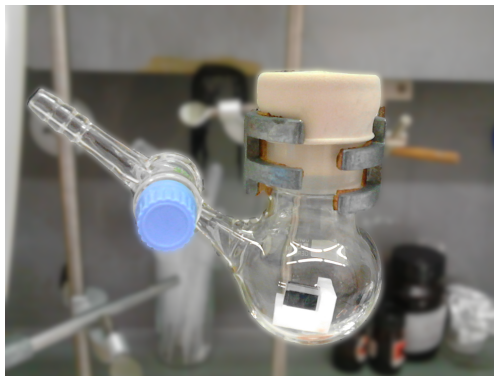
Figure B.1.: Sample arrangement: Patterned CNMs plugged into a self-built Teflon holder and placed into a schlenk flask, which was equipped with a septum.
