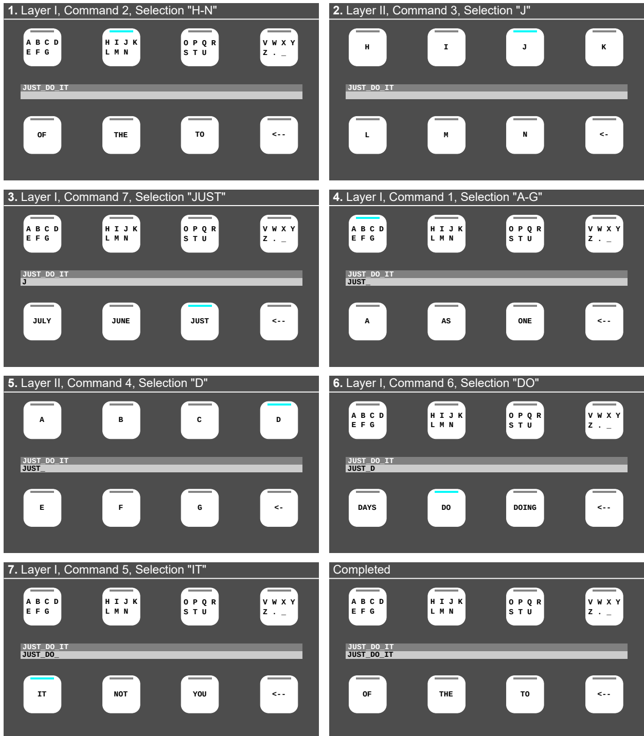
Figure 5.3: GUI of the dictionary-driven c-VEP spelling application. A participant was spelling the sentence "JUST DO IT". The selection of individual letters required two steps: First, the group containing the character needed to be selected (Layer I), and second, the box with the desired character needed to be selected (Layer II). In total, seven selections were required to complete the sentence (10 characters). Due to the sliding time window mechanism, there were no time constraints for selections.
