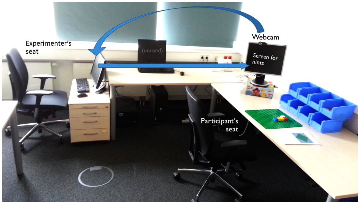
Figure 7.3: Lab setup for the Duplo assembly study. A webcam live stream of the assembly area enabled the experimenter to observe participants' actions and intervene on errors by triggering an auditory signal and displaying the correct action on a screen next to the assembly area.
