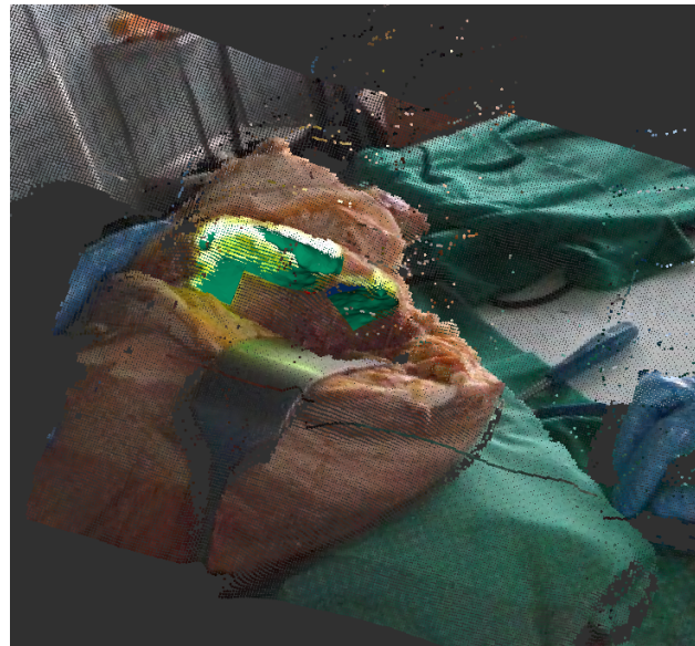
Figure 3. Recorded rosbag of test surgery on corpse shows depth image with a registered color image. The projection on the bone can be seen in light green, the current tracking output in green.
