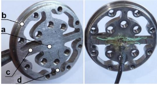
Figure 2: Sensor structure (left) - inner mounting part (a), outer mounting hoop (b), sensor beams (c), short beams (d); strain gauges glued onto the sensor (right).
