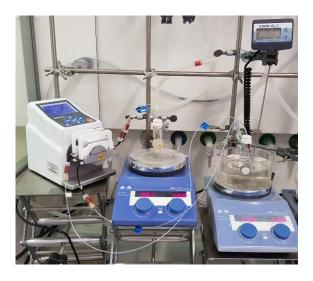
**Figure 21:** Foto of the used flow set up showing the two reactions in each flask (**Flask 1** left for the biotransformation, **Flask2** right for the racemization and isomerization) connected to a peristaltic pump.
