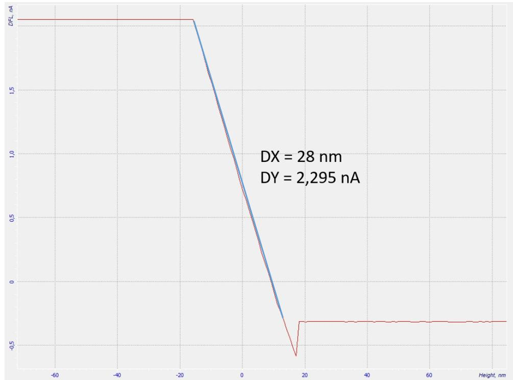
**Figure 5.6.:** Reference force curve recorded on the substrate. The slope of the blue curve was used to determine the cantilever bending per change in the photo detector signal.
