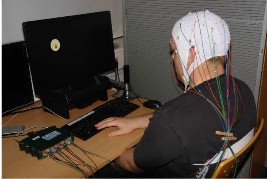
FIGURE 6.3: Example of how the recording sensors were set up. The eyetracker is placed below the interaction screen and the EEG is placed next to the subject. The interaction scene seen on the screen is not related to this presented work.
