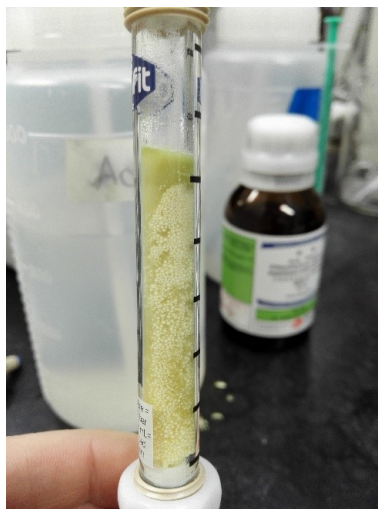
Figure 7.3: Particle separation of DualPore silica and CAL-B after a reaction (approximately 5 h operating time).
