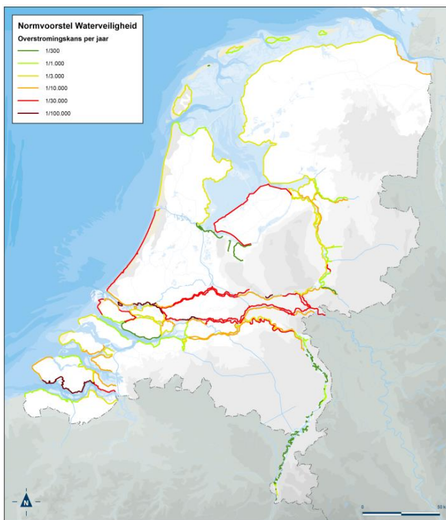
Fig. 2: New proposed safety standards in the Netherlands, based on acceptable probabilities of flooding (source: DELTAPROGRAMMA, 2014)
