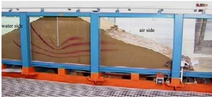
Fig. 2: A physical model dam with slides on the air side (Aigner, 2004)
