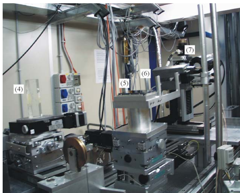
Figure 3-2 SYRMEP beam line ELETTRA/Trieste in DEI operation (4) Sample stage (5) Si analyser crystal (6) Second ion chamber (7) CCD camera
